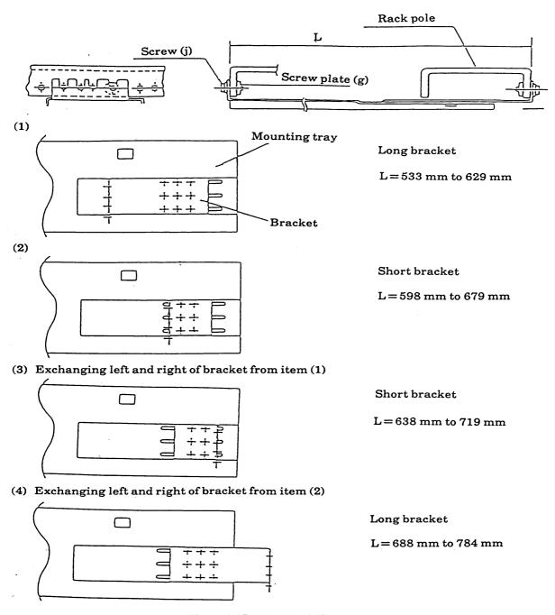
Figure 1-15. Bracket Adjustment
